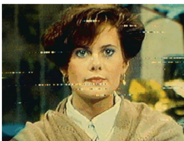
Picture 7: Electrical Interference -- low noise
