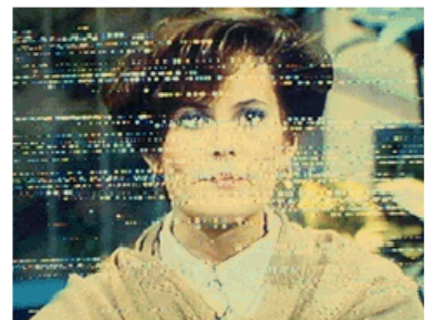
Picture 6: Electrical Interference -- very noisy (hair dryer)
